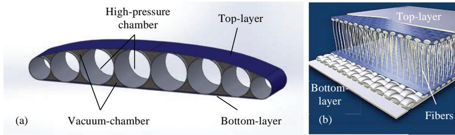
Fig. 2. (a) VacuuAir-construction; (b) Dropstitch-construction [4]
