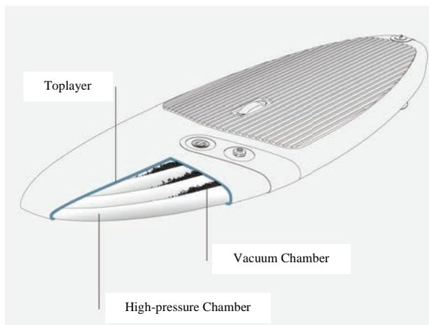
Fig. 3. VacuuAir-construction: chamber arrangement
